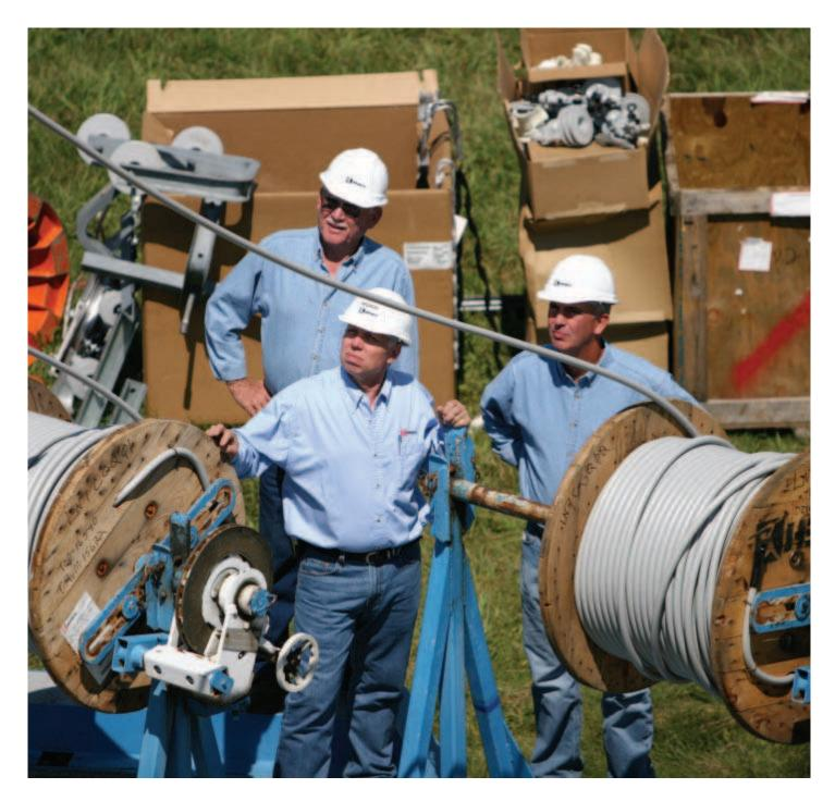
It's all in the kit: Hendrix Wire & Cable have developed a Kitting Solution to complement the Spacer Cable System. It ensures cables are cut to length for a specific job, thereby reducing scrap and installation time. There are no short lengths left on the reels, less set ups on the reel trailers and less splicing.
