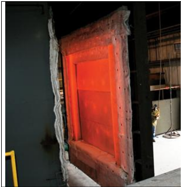
Refractory concrete firewall test
